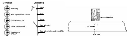
Fasten AbsoluteTrim™ from one end to the other end. Do not nail towards the center from both ends.
