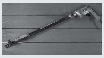
Some Trex recommended deck fasteners are compatible with screw guns. Refer to the recommended fasteners page for more information.
