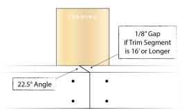
the trim/fascia segment is 16' or longer leave a 1/8" gap. Scarf joint cuts at a 22.5° angle. Double nail joints on both sides as shown here. It is highly recommended the joint be caulked with a high quality, flexible exterior sealant (OSI Quad Max or equivalent).
